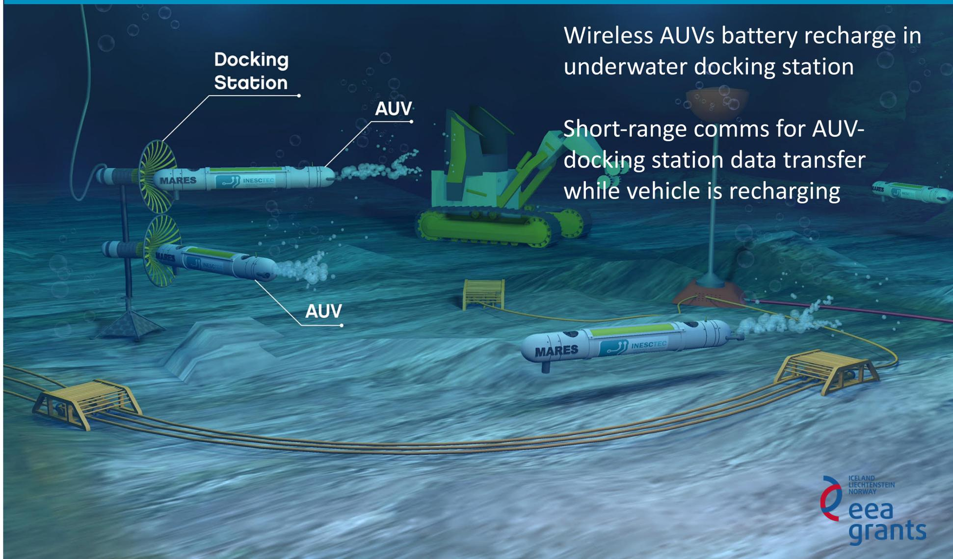
Wireless AUVs battery recharge in underwater docking station
