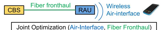
The hybrid optical-wireless link that is configured when cascading the fibre fronthaul and air interface becomes and Amplify-and-Forward (AF) relaying system
