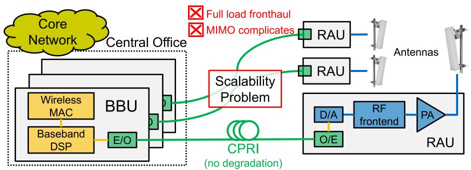
CPRI transports digitalized I-Q samples (plus sync, control and management) that <u>expand</u> the data rate and introduce <u>delay</u>
